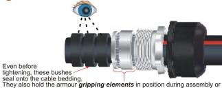
They also hold the armour *gripping elements* in position during assembly or during inspections. The gland seals are rendered fully inspectable!
